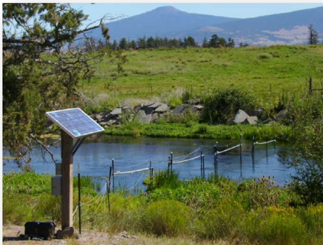
Pit tag antennae in the upper Shasta River
