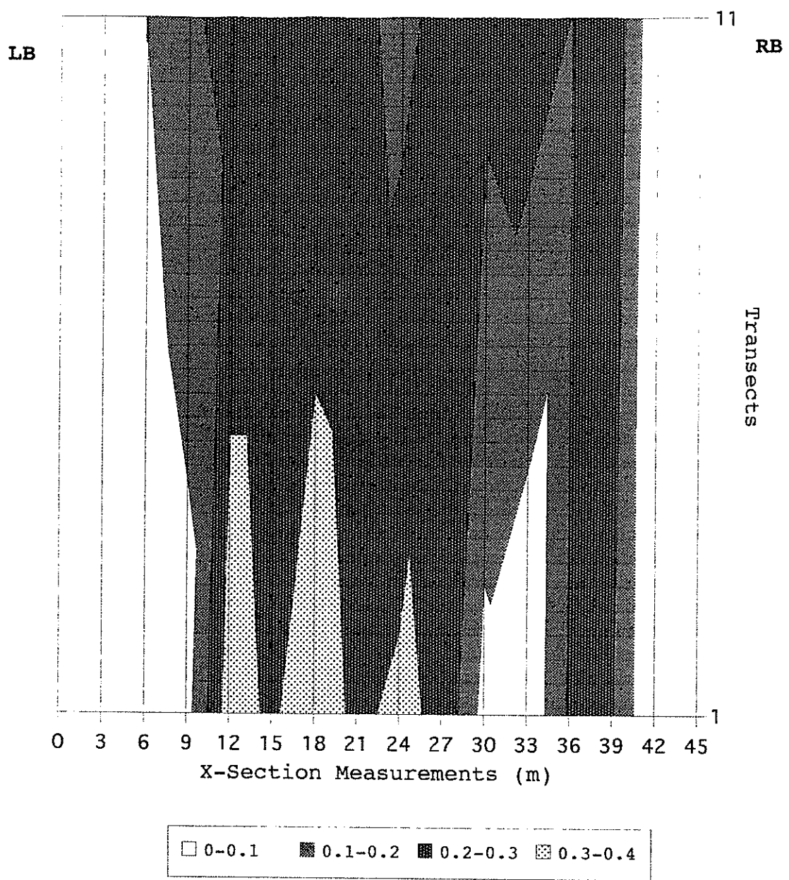
Appendix F. Study Unit #2 mean water velocity profile. Water velocity was measured along the first and last transects of the unit. These measurements were expanded to represent water velocity throughout the unit.
